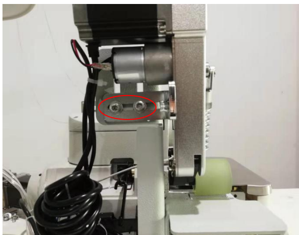
M6 螺丝固定上下轮子贴紧
